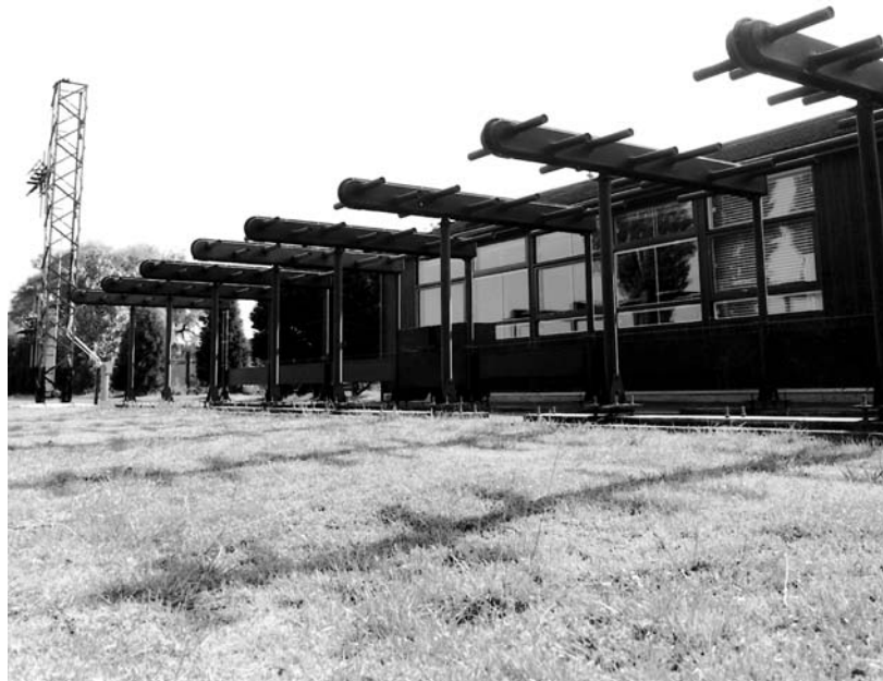
Fig 4-7: The ILS localiser aerial (note the photograph shows a technicians training setup. There would be no office block at a real site)
